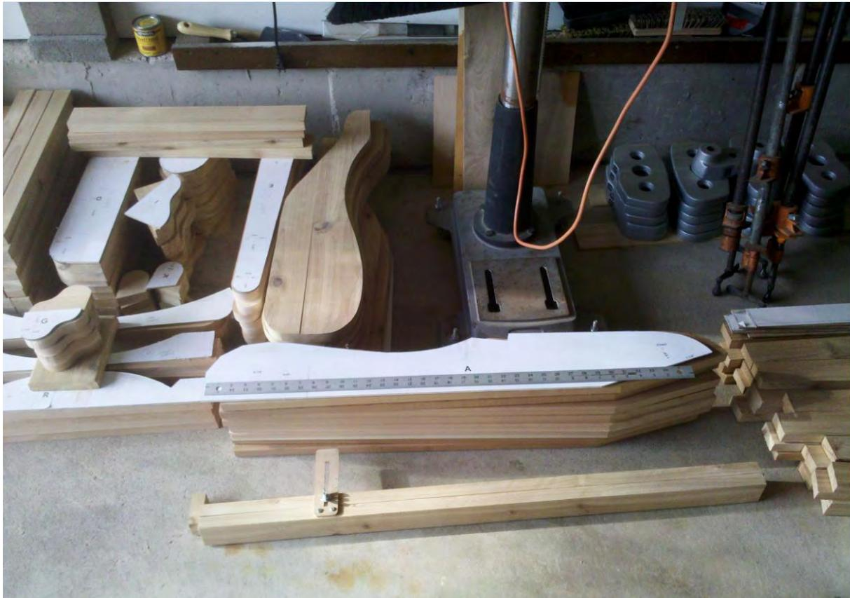
Most of the pieces had to be "paired" for grain and matching hole location. Then identified as part of Chair 1, 2, 3, and 4 early in the process. Sharpie to the rescue! It took about a week to drill all of the necessary holes. Below are the Forstner bits required and the Stain [Sikkens Cetol 1, Dark Oak].
