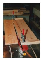
Trace part I onto the board, and trim off one side as shown. Reverse the traced pattern, and cut off the next piece. Cut all back slats to the length of the middle slat part I, then trace on the other patterns for J, K & L, and trim at the band saw.
