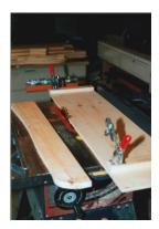
Made from a scrap of 1/2" x 9 1/2" x 39" veneered fibreboard, attach a matching length of 3/4" x 9 1/2" x 2" scrap to the top of the sled. Screw on an adjustable toggle clamp to the left side. At the bottom of the sled, attach a matching board with a clamp, 2" longer than Part E, the back support.
