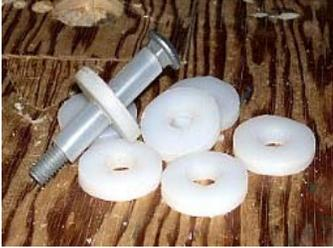
**8** - Here you can see the final assembly of the bolt, plastic waterline and plastic washer ready for assembly.
