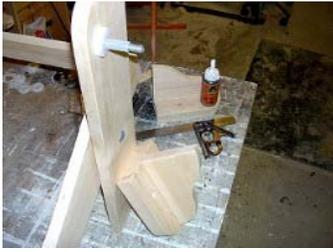
**5** - Push the bolt and tubing from the inside of part **D**. Then add the washer in between and push the assembled part **H&I** in place. Add the flat washer, then lock washer and tighten the nut. The tops of parts **D & H&I** should be flush and square. If not, sand both sides of the chair, so they are exactly the same height.
