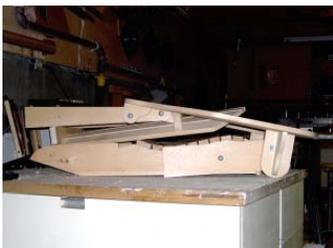
**16** - You can now fold your chair by pushing forward at the top of the back. The front legs should fold forward and the chair will collapse. To open again, put your foot on the back dowel and pull up on the back. The chair will lock into the slot in the side panels in the reclined position. Pull back on the top dowel or the back supports to put the chair in the regular position.
