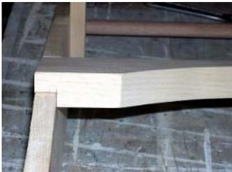
**9** - After cutting out part **M**, you need to rabbet the ends so the part fits flush to the top of parts **A**. Cut out a 1/2" deep x 3/4" wide (1.25cm x 1.9cm) rabbet in the underside being sure that it also fits easily into place between the side panels **A**.
