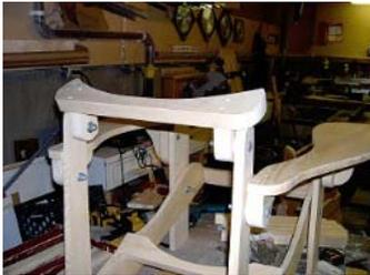
**8** - Assemble the back support pivot parts **K** in the upper holes on the inside of back supports **E**. Be sure that the tops are angled towards the back of the chair. Center the back support part **L** on the pivots, drill pilot holes, **glue** and screw in place with two 2" (5.1cm) screws into each pivot.
