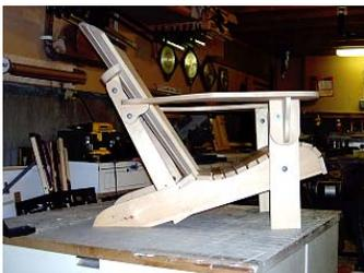
**15** - To recline the back, sit in the chair, reach your arms back around the back slats, grab the back supports **E**, and pull forward. To put it back in the upright position, reverse the process. Check to be sure there is no binding at part **R**. The supports **E**, should fold against the back of part **M**. The front legs may tilt back slightly when you lean back. If you don't want the chair to recline without getting out of the chair, add another dowel in front of dowel
