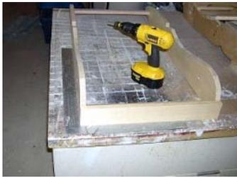
**1** -Begin assembly by cutting the dowel part **B** to length and screwing in place between parts **A**, the side panels, with 2" (5.1cm) screws. Next attach the front slat **C**, with two 1/58" (4.2cm) screws on each side, to the front edges of parts **A**, flush with the bottom edge, or with a 1/4" overlap as I prefer. This will give you a carcass to work with. Check for square by measuring corner to corner, both ways. If the carcass is not square, the chair will not fold.
