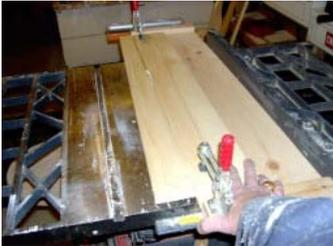
**2** - A taper jig on the table saw, works best for the back slats and back supports E. A shop built sled is the quickest, easiest and safest taper jig. Use a scrap length of 6" (15.8 cm) wide plywood, longer than back slat **N**, and fasten clamps at each end. Line up the pattern line to the edge of the jig, using an adjustable square, and run it through the blade.
