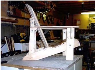
**14.** The chair is now assembled, and ready for finishing. If you are plugging the screw holes, I recommend a tapered plug cutter, like the Veritas Cutter from Lee Valley Tools or the hex shank tapered cutter from Rockler. Glue the plugs in place with exterior waterproof glue, let dry, then cut off the excess with a chisel or Japanese saw. The rest can be sanded smooth with a random orbital sander. Touch up the plugs with primer, if painting the chair.
