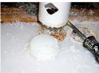
**6** - Using the UHCW plastic, make 8 washers using the 1 5/8" (4 cm) hole saw. The Lee Valley plastic is already 1/4" ( 6.5mm), but if you buy 3/8" (9.5mm) plastic jig stock at Rockler, rip or plane it to size. Use a cutting blade to trim off the plastic burrs to make the washer smooth.
