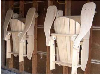
**17** - To finish the chair, disassemble it at the bolt positions. You will then be able to finish it much easier. After reassembling the chair, use locktite on the nuts, tighten and then back off slightly.
