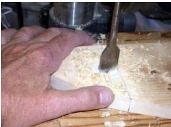
**5** - Using a 7/8" (2.2cm) spade or Forstner bit, drill the 1/4" (6.5mm) deep holes for the dowels in parts **A** & **E**. **NOTE:** Be sure to drill the holes on the **INSIDE** of each part. The back supports, parts **E**, are square at the front & angled at the back, so lay them together, then open like a book, and mark the hole locations on the inside.
