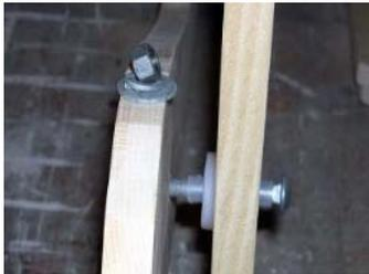
**2** - Next, bolt on the front legs **D**, on the **OUTSIDE** of parts **A**. Cut a piece of tubing to 1 5/8" (4.15cm) and slide it over the bolt to the square head under the crown. Push the bolt through the lower hole of part **D** being sure that the curve at the top faces the back of the chair. Add the plastic washer, then push the bolt through the front hole of part **A**. Double check the length of the tubing to be sure it doesn't protrude past the inside of part **A**.
