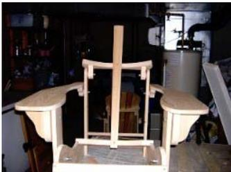
**10** - The back pieces can now be assembled, starting with the middle slat **N**, centered at the top on part **L**, and at the bottom, in the curve on part **M**. Overhang 5/8" (1.6cm) below the bottom of support **M**. Use one 1 5/8" (4.2cm) screw at the top and bottom of each slat, being sure not to set the screws too deep.
